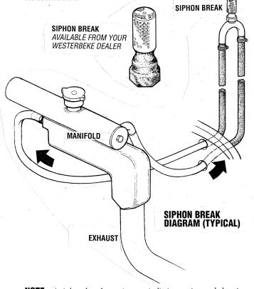
**NOTE:** A siphon-break requires periodic inspection and cleaning to ensure proper operation. Failure to properly maintain a siphon-break can result in severe engine damage. Consult the siphon-break manufacturer for a proper maintenance schedule.
