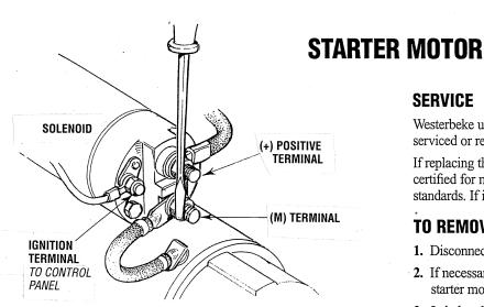
Test again by jumping the two large terminal studs. Hold the screwdriver blade firmly between the studs. Do not allow the screwdriver blade to touch the solenoid or starter casing, this would cause a short.
