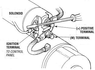
If nothing at all happens the solenoid isn't getting current. Check the battery isolation switch and inspect the wiring connections. It is also possible that the solenoid is defective.
