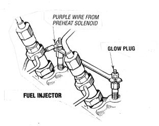
Re-install the plugs in the engine and test them again. The plugs should get very hot (at the terminal end) within 20 to 25 seconds. If the plugs don't heat up quickly, check for a short circuit. When reinstalling the glow plugs, use anti-seize compound on the threads.
